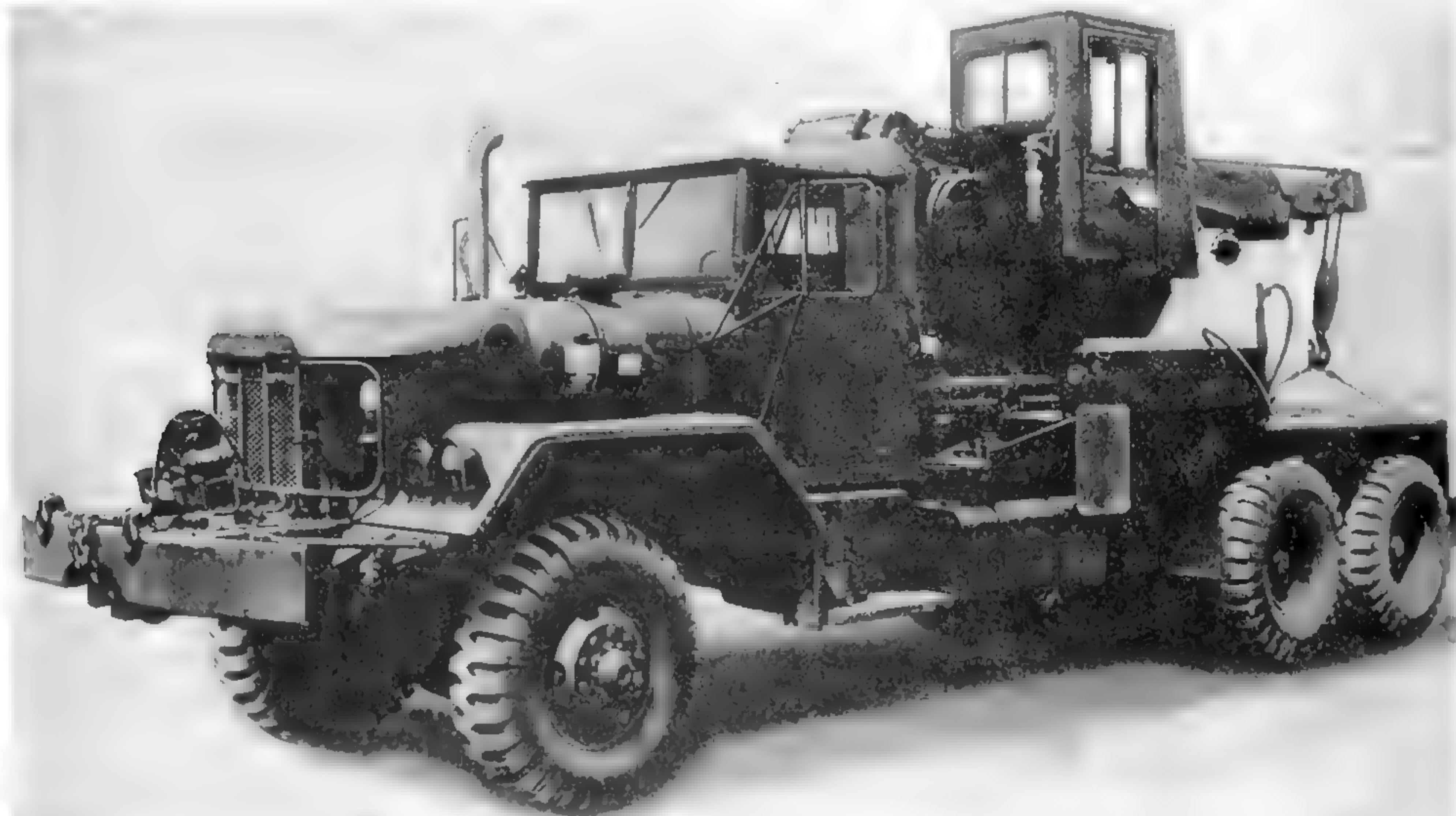
The crane operator's station of the M819 could be fully enclosed with a hard top kit. In the absence of the hardtop kit, a canvas tarpaulin and bows were provided for the crane operator. (U.S. Army photo)
